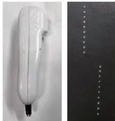
FIGURE 4. A home-use, non-ablative 1470 nm fractional laser demo system (200g, 210 × 55 × 60 mm 3 ) at Focuslight and the spots it generates.
